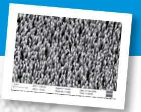
SEM image of Vanadium-doped zinc oxide nanostructures
